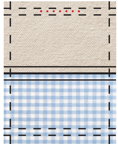
IRON THE DOUBLE FOLD TOP AND BOTTOM INWARD WITH NOSE PIECE INTO PLACE
